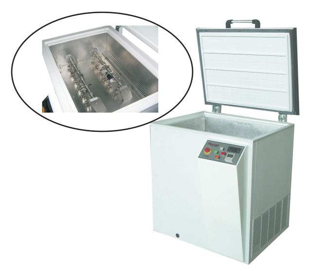
"BALLY" flexing machine with 12 stations and cold chamber
